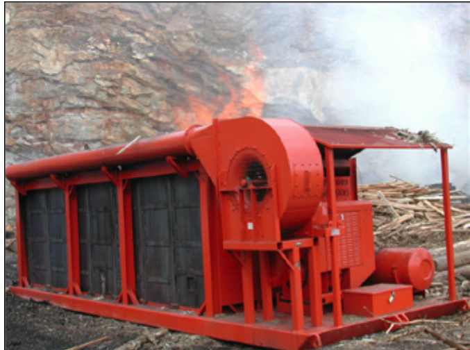
Fig. 1. An air curtain destructor being used to destroy turkey carcasses infected with low pathogenic avian influenza in Virginia in 2002 (Source: Gary Flory).
