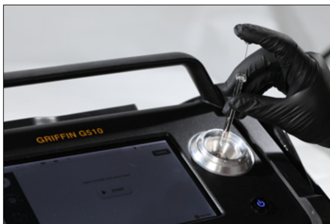
Fig. 2. Direct syringe injection performed on GC-MS (Source: FLIR Systems Inc., 2017).
