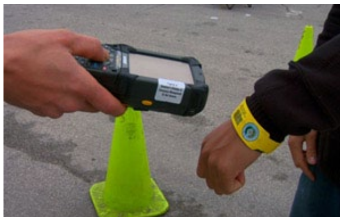
Barcode scanning is an effective technique at lower volume processing sites. Each Texas band is unique and allows the four Texas Emergency Tracking Network systems to work in tandem without duplication of individuals.
